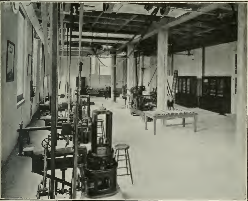
FIG. 2.—TIMBER-TESTING LABORATORY, SHOWING THE SMALL TESTING MACHINES.
