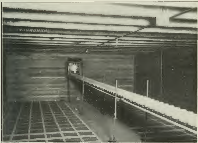
FIG. 2.—PRECOOLING ROOM IN AN ORANGE-PACKING HOUSE AT EAST HIGHLANDS, CAL., SHOWING ROLLER CONVEYOR FOR CARRYING THE PACKED BOXES OF FRUIT INTO THE PRECOOLING ROOM.
