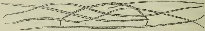
FIG. 17.—Rice-straw fibers. Though comparatively short, these are strong and felt well. (Enlarged 71 times.)
