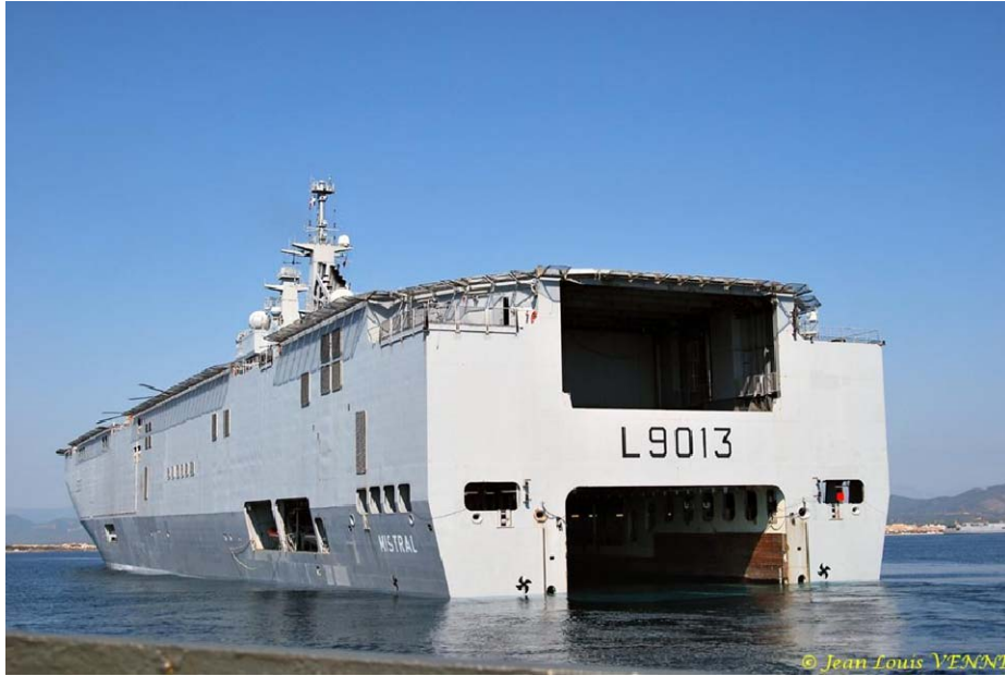
Figure 16. Picture showing the open well deck of Mistral (From Jean Louis Venne)
