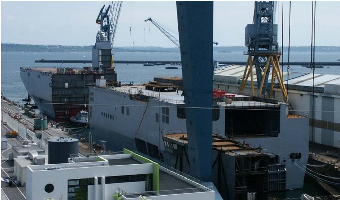
Figure 7. Mating of the forward and aft sections of the Mistral (From Yannick Le Bris, 2004)
