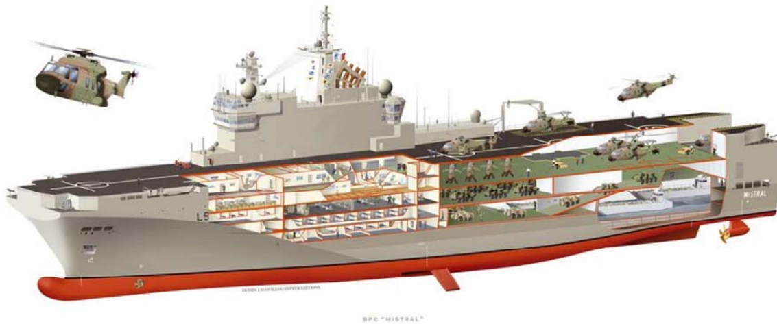
Figure 15. Internal cutaway of Mistral showing deck layout. Also note propulsion system (from enibule.com)
