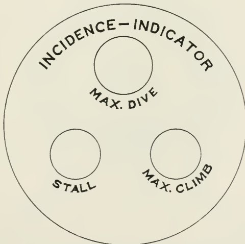
Fig. 60—Indicating dial connected to incidence indicator shown in Fig. 59
