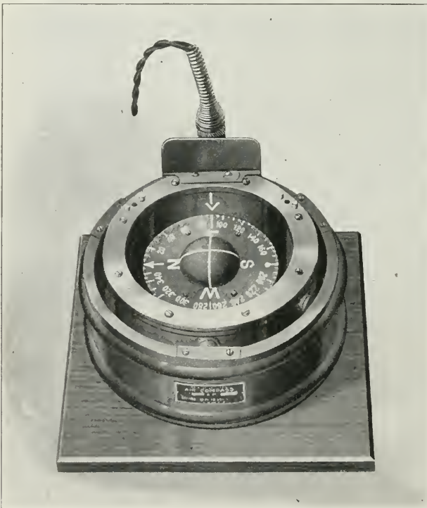
Fig. 53—Creagh Osborne type of airplane compass
