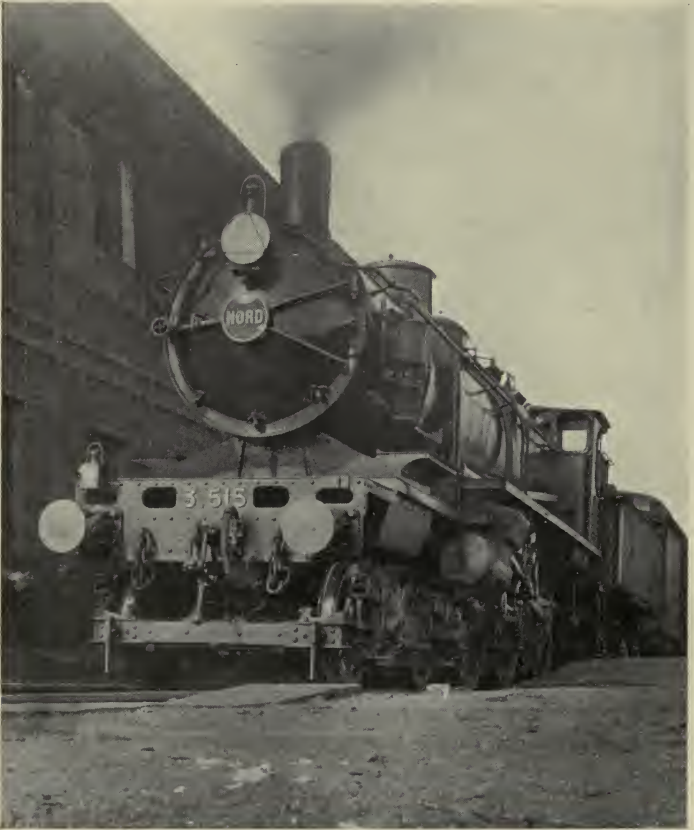
4-6-0 FOUR-CYLINDER COMPOUND ENGINE (NORD).
