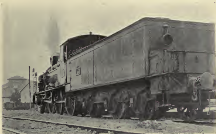
P.L.M. FOUR-CYLINDER COMPOUND EXPRESS ENGINE 2608 (ANOTHER VIEW).
