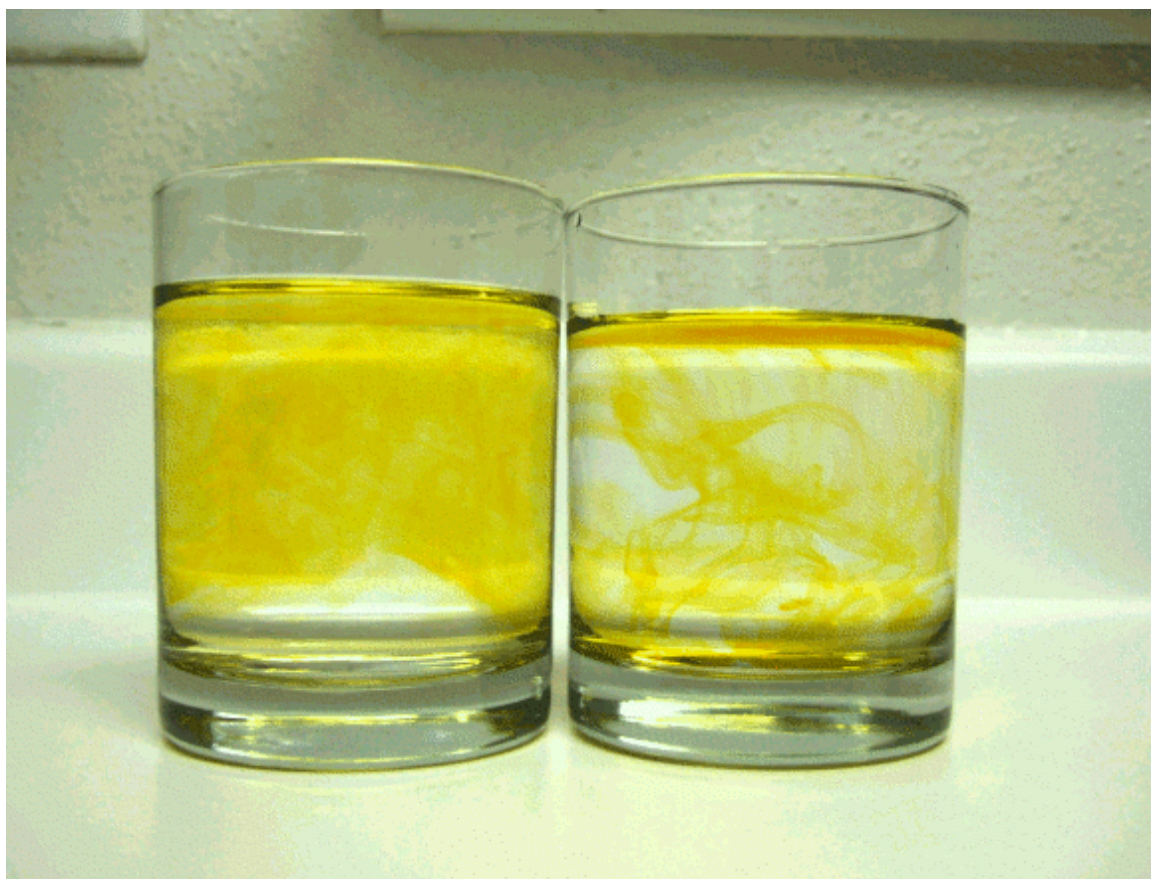
Figure 123 Diffusion is the chaotic mixing of fluids. The jar on the left has warmer water.
