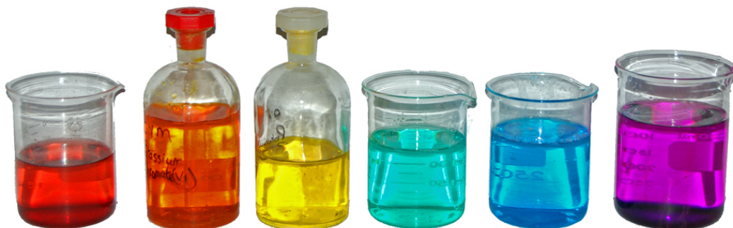
Figure 175 Left to right: cobalt(II) nitrate (red); potassium dichromate (orange); potassium chromate (yellow); nickel(II) chloride (green); copper(II) sulfate (blue); potassium permanganate (purple).
