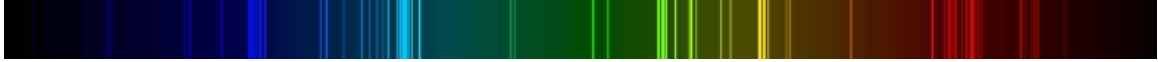
Figure 23 The emission spectrum of nitrogen gas. The spectral lines occur at specific wavelengths, showing the particle behavior of light.
