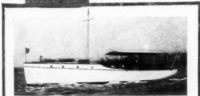
40-ft. Elco Cruiser. Sleeps Seven. 20 horse power Standard Gasoline Engine. Designed for ocean cruising
