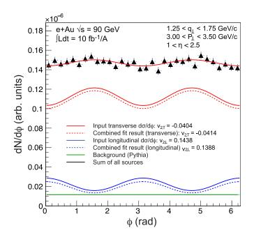
FIG. 14. Result of a fit of combined signal and background to a data sample obtained in  $\sqrt{s} = 90$  GeV *e*+A collisions with an integrated luminosity of 10 fb<sup>-1</sup>/nucleon. For details see text.
