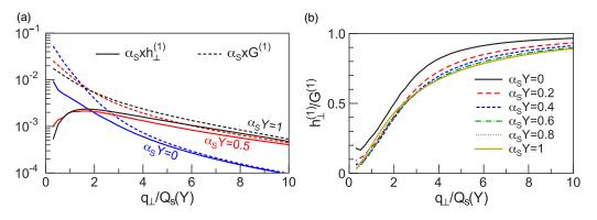
FIG. 1.  $xG^{(1)}(x, q_{\perp}^2)$  and  $xh^{(1)}(x, q_{\perp}^2)$  WW gluon distributions versus transverse momentum  $q_{\perp}$  at different rapidities  $Y = \log x_0/x$ .  $Q_s(Y)$  is the saturation momentum. The curves correspond to evolution at fixed  $\alpha_s$  [19].
