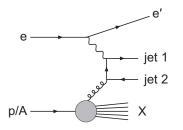
FIG. 10. Photon-gluon fusion processes that contributes to the 2+1 jet signal cross section.
