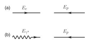
FIG. 2. The reference frames: (a) The laboratory frame. In the laboratory frame, the electron and the proton have zero transverse momenta; the energy of the electron (proton) is  $E_e$  ( $E_p$ ). (b) The analysis frame. Here, the virtual photon and the proton have zero transverse momenta; the energy of the proton is the same as in the laboratory frame, equal to  $E_p$ . The energy of the virtual photon is  $E_{\gamma^*} = (q^+ + q^-)/\sqrt{2}$ , see Eqs. (23) and (24).
