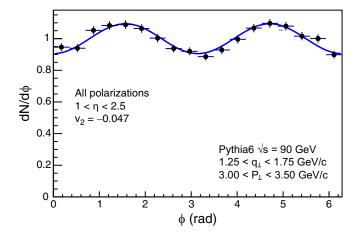
FIG. 12. Azimuthal asymmetry in reconstructed dijet events from PYTHIA caused by the limited  $\eta$  acceptance.
