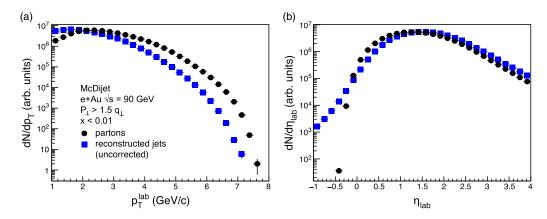
FIG. 6.  $p_T$  and  $\eta$  distributions of partons (filled circles) and reconstructed jets (filled squares) in the laboratory frame. The jet spectra are uncorrected.
