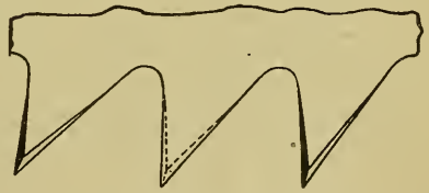
FIG. 196.—TEETH OF RIP SAW (CIRCULAR).
