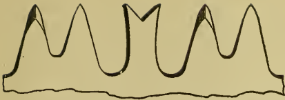
FIG. 195.—TEETH OF TWO-MAN CROSS-CUT SAW.
