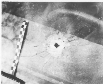
Bullet hole in windshield, in front of steering wheel. Measuring tape on left rests on windshield wiper.
