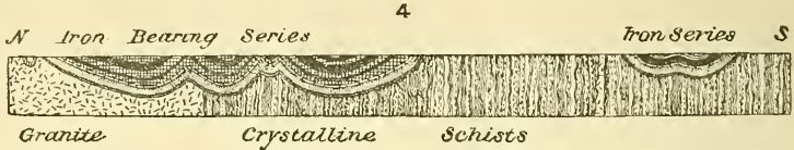
FIG. 4.—Generalized ideal section of the Marquette region in the vicinity of Ishpeming. In part after Brooks. Scale, 3 miles to the inch.
