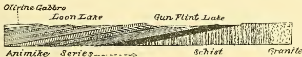
FIG. 9.—Section across Gunflint and Loon Lakes, on the national boundary line. Scale 1\frac{1}{2} miles to the inch. Designed to show the relation of the Animiké series to the older schists and granite, and to the newer Keweenawan gabbro. Scale 1 mile to the inch. The black bed at the base of the Animiké is the ferruginous horizon. The remainder of the Animiké in the section is composed of slates and slaty quartzites with interstratified greenstones.
