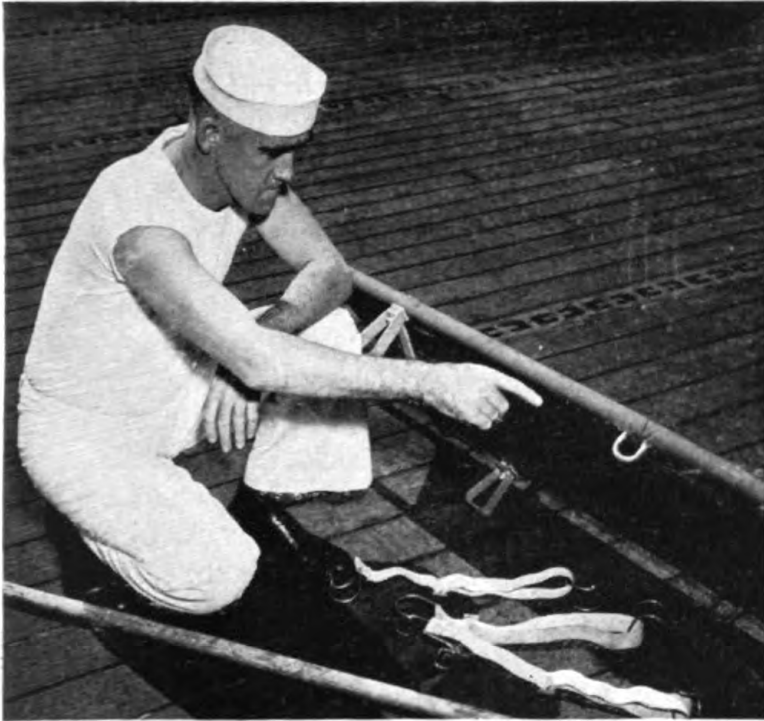
2. Showing eye to accommodate 1-inch pipe welded to frame of Army-type litter.
