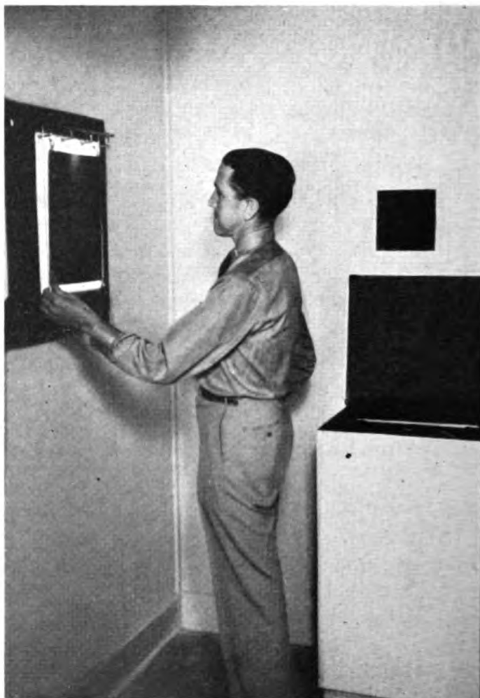
4. Wet-film viewing room in use.
