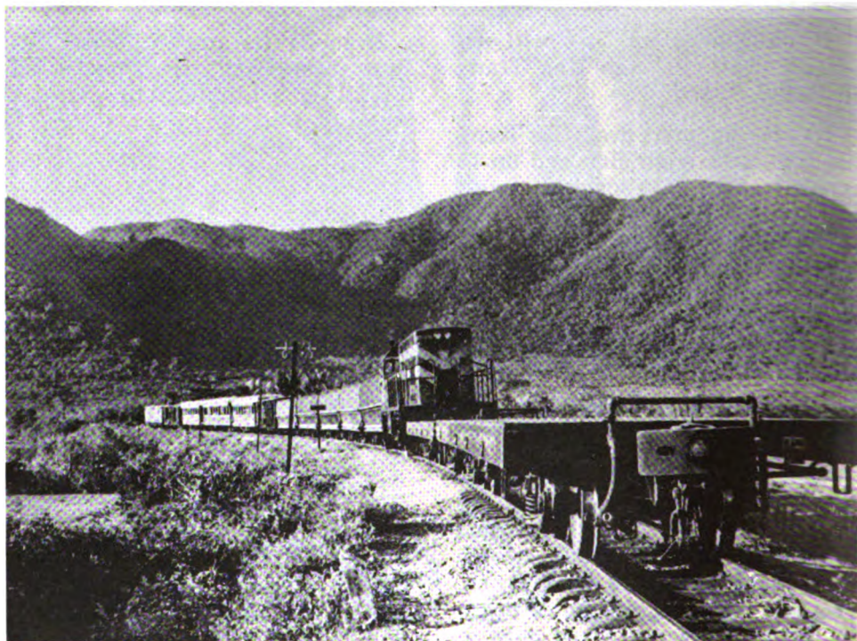
South of Phu Cat, this train runs with flatcars hooked ahead of die to detonate any land mines the Viet Cong may have placed on the tracks.
