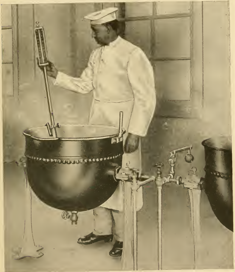
FIG. 95.—A steam-jacketed preserving kettle. (Heinz Company.) Note use of thermometer and arm and ball weight valve to control steam pressure.
