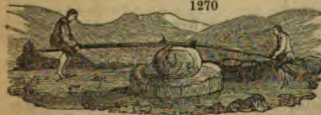
Fig. 1270, represents the rude grinding apparatus used at the lavaderos in Chile. The streamlet of water conveyed to the hut of the gold washer
