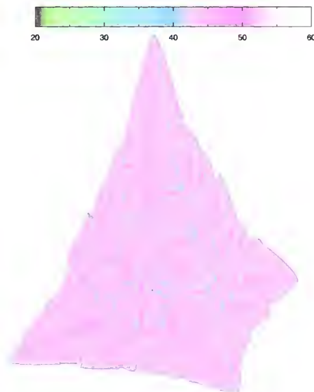
Fig. 17. A 3D dendrite from a simulation over a grid of 300^3 points. The color bar shows the coding of the relative concentration of the metals in the dendrite. The color coding ranges from concentrations of 20 % to 60 %.
