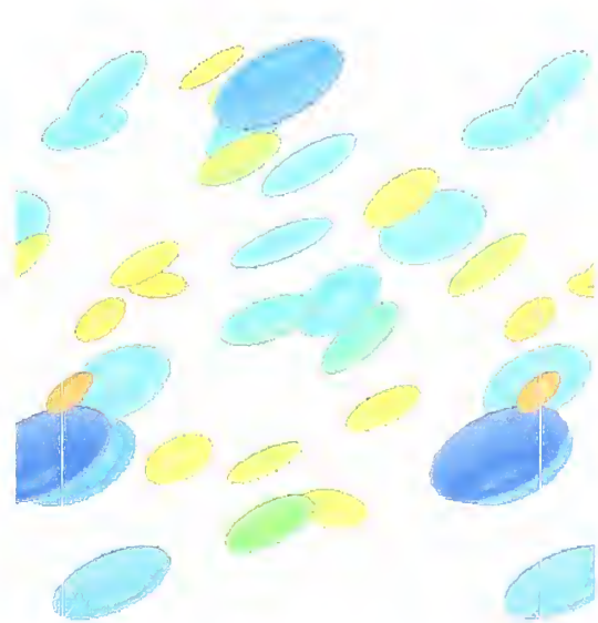
Fig. 8. Motion of twenty eight ellipsoidal inclusions, of size varying up to a factor of two, subject to shear. Note that the Jefferys orbits are suppressed due to hydrodynamic interactions between ellipsoids.
