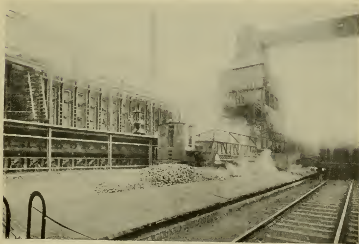
2. BY-PRODUCT COKE OVENS, SHOWING THE COKE BEING REMOVED FROM AN OVEN TO THE QUENCHING CAR
