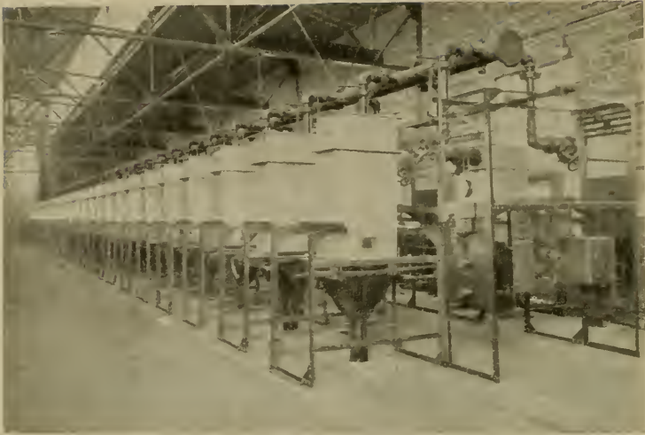
1. CATALYTIC PLATINUM BURNERS IN THE AMMONIA OXIDATION BUILDING AT THE UNITED STATES NITRATE PLANT No. 2
