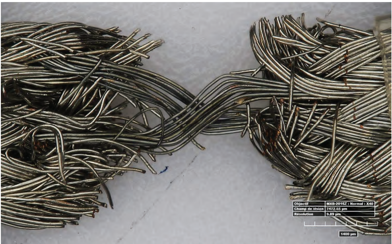
Sample after test – Light coloration of remaining wires
