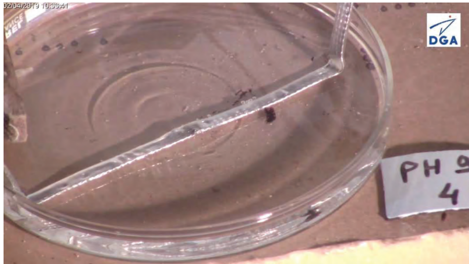
Figure 25 : Serial arc test in solution – HS4 sample 4% in pH9 without PR
