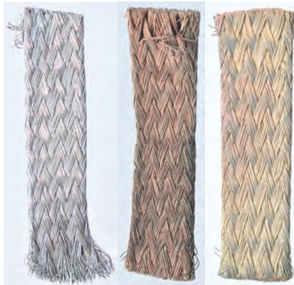
Samples immersed from left to right in HBr - HF - H 2 SO 4
