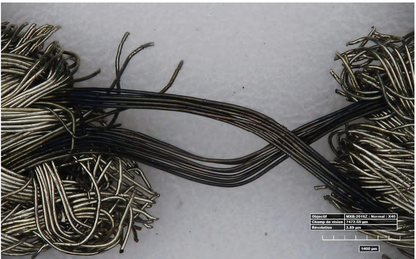
Sample after test – Significant coloration of remaining wires
