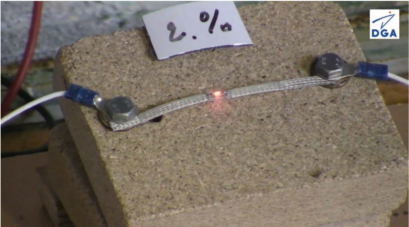
Red glowing braid just before arcing
