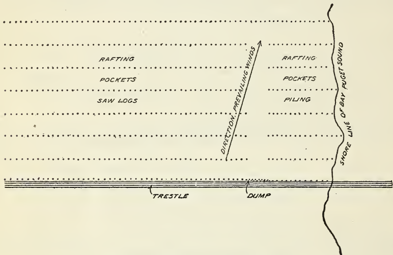
FIG. 83.—Booming and rafting works.
