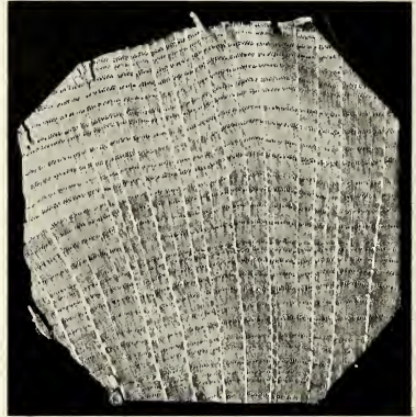
THE ANNUAL RINGS AND RAYS OF AN OAK. (A PIECE OF OAK FROM SOUTH CAROLINA.)
