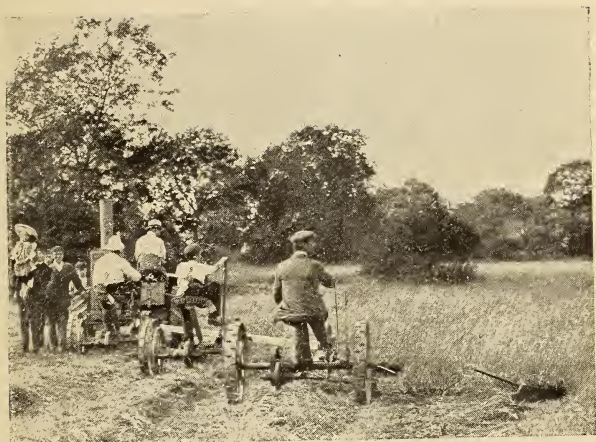
IVEL MOTOR HAULING THREE REAPING MACHINES, CUTTING A TOTAL WIDTH OF 18 FT. EIGHT ACRES WERE CUT IN TWO HOURS. SIX HORSES REPLACED BY ONE MOTOR
