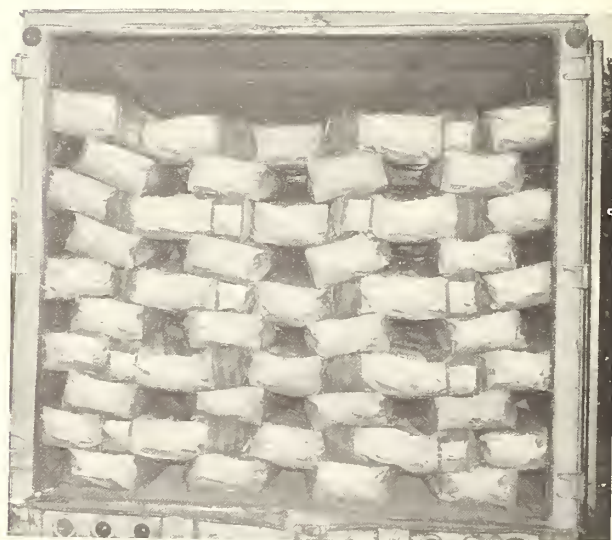
FIGURE 7.—Airflow pattern No. 3 using 50-pound tape-closure master paper sacks, each of which contains five 10-pound bags. This pattern is designed for use in wide trucks with header stack as shown in figure 6(A).
