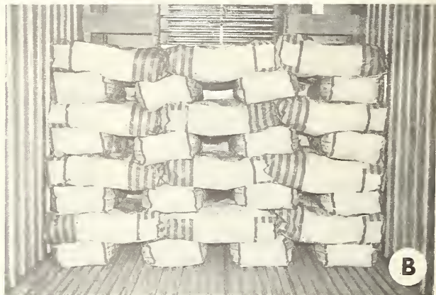
FIGURE 6.—Airflow pattern No. 2 using 50-pound tape-closure master paper sacks. This pattern is designed for use in narrow trucks. (A) First or header stack. (B) All subsequent stacks.
