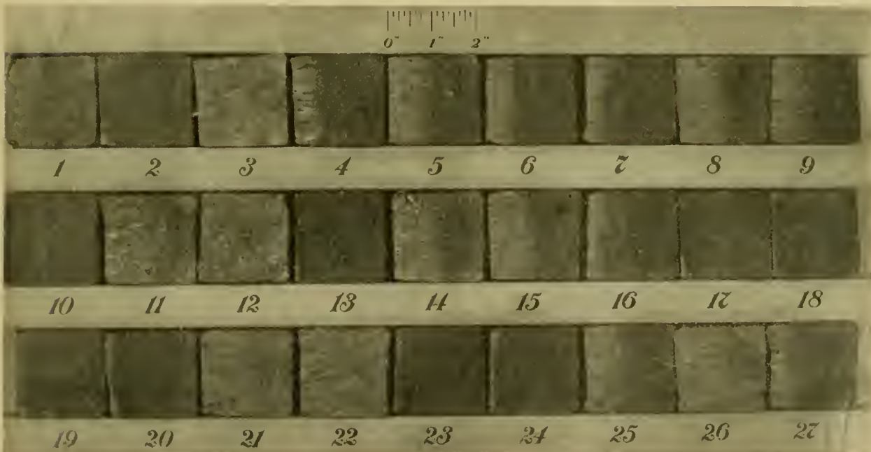
Fig. 4.—Showing Appearance of Fractures of Chilled Test Bars.
