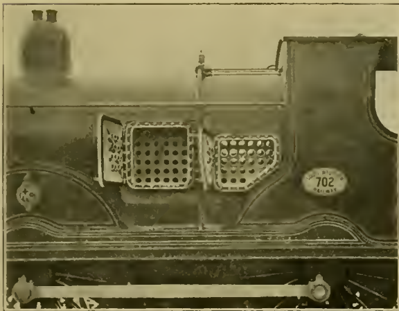
Side View, Showing Ends of Tubes.
