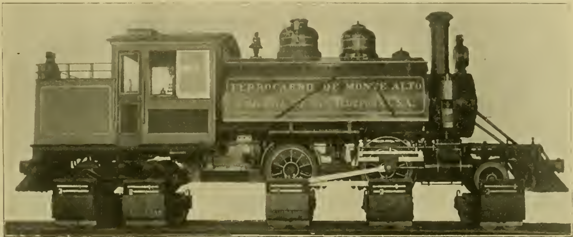
A Locomotive Mounted on the Scales.
