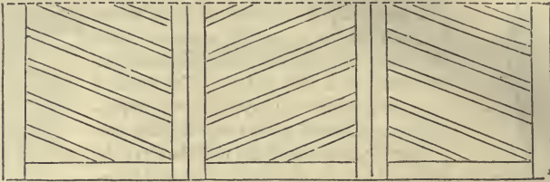
Fig. 133. Vertical profile of part of a ridge and furrow roof.
