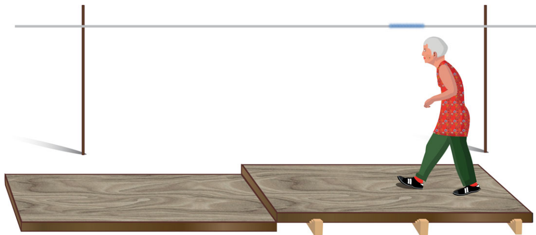
Figure 1. Illustration of the experimental set-up. Participants were asked to step down at the end of the first platform. The step height was adjustable and ranged from 0.025 to 0.15 m. The participant was instructed to adopt a walking speed of 1.1 \text{ m s}^{-1} , as indicated by an LED strip alongside the platform.
