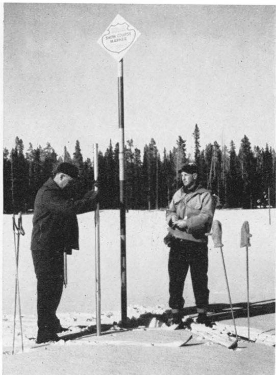
Out on the course a snow sample is taken by thrusting the Federal sampler—a 1 \frac{3}{4} -inch hollow, aluminum-alloy tube—down through many feet of snow to the ground beneath.
