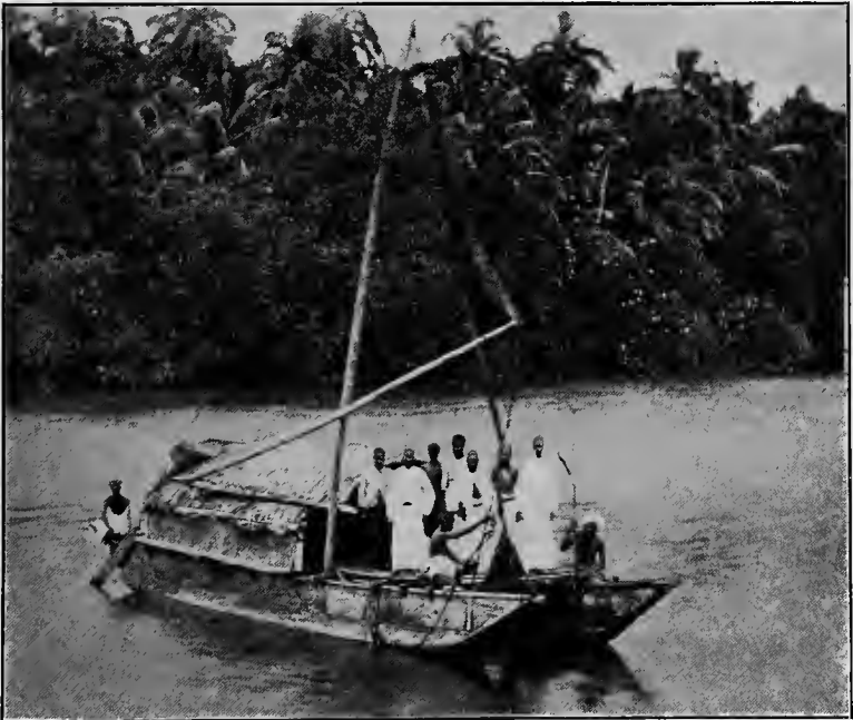
Modern double canoe with deck-structure, of the sangāra type; in general use in South India, Ceylon, and the Eastern Archipelago.
