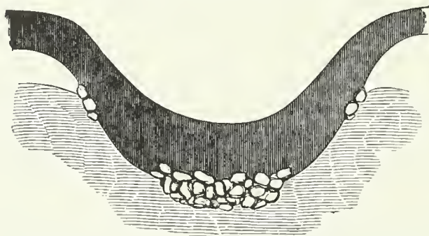
SECTION THROUGH ONE OF THE PITS AT WEYBOURNE, SHOWING METHOD OF CONSTRUCTION.
