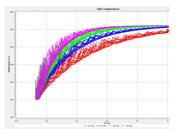
Figure 25. Tube Temperatures for Pressure Driven Boundry Conditions
