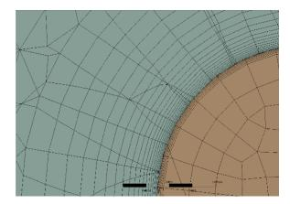
Figure 19. Detail of Mesh 4 Inflation Layer
