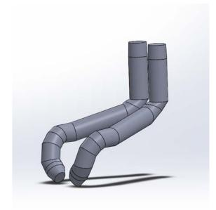
Figure 8. Exhaust Ducts by VanDenBerg. Source: [1].
