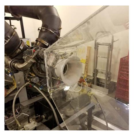
Figure 6. Bell Mouth Installed on Engine
