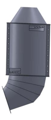
Figure 9. Assembled Model of Duct with Heat Exchanger Coils
