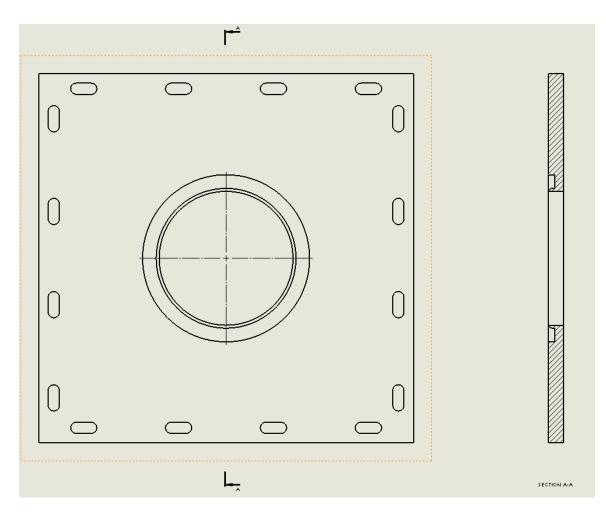
Figure 7. Flange Model Cross Section
