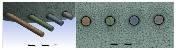
Note the inflation layers surrounding the tubes and the size of the elements in the green tube (left). Increasing the size would reduce the mesh size by  $\sim$ 1 million nodes.
