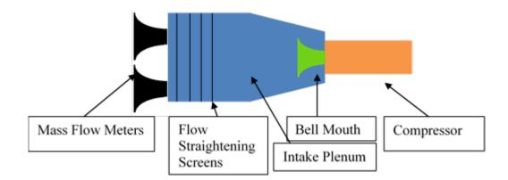
Figure 4. Schematic Drawing of Air Intake System
