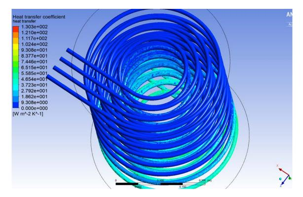
Figure 26. Heat Transfer Coefficient on Bottom of Coils
