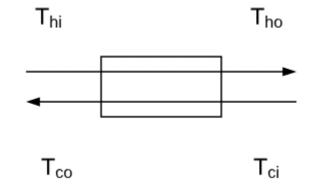
$$\dot{m}_{exhaust} = .7 / 5 = 0.14 \implies q_{exhaust} = 9.24 \, kW$$
