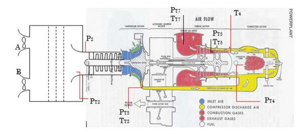
Figure 2. Schematic of the T63-A-720 Engine<sup>1</sup>
