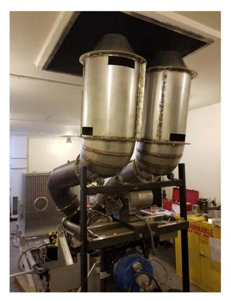
Figure 10. Installed Heat Exchanger Duct
