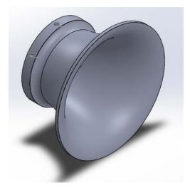
Figure 5. Bell Mouth SolidWorks Model
