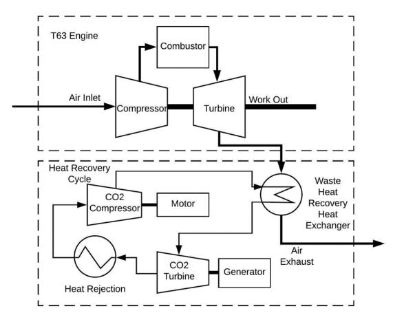
Figure 1. Waste Heat Recovery System Schematic
