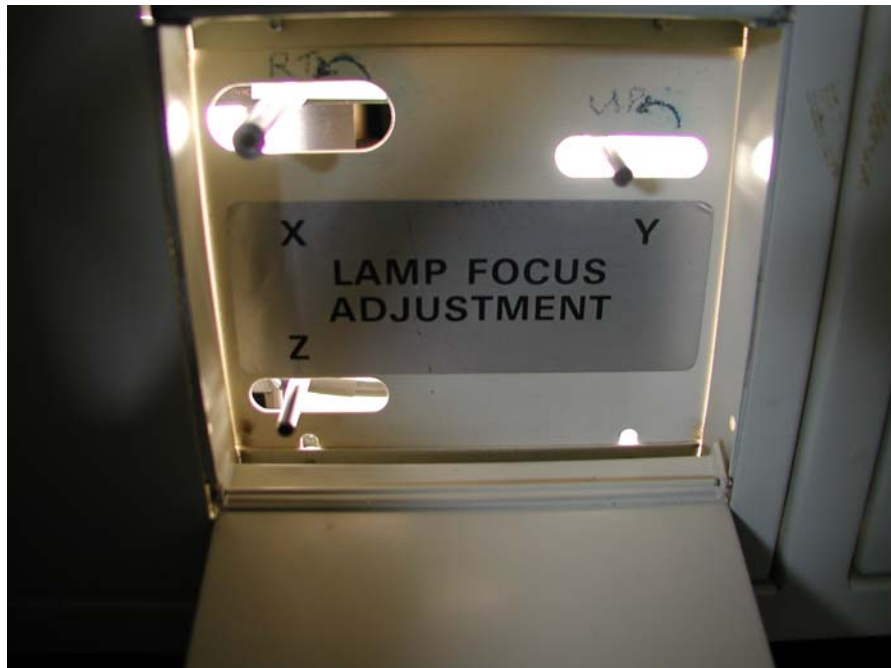
Figure 35. X-Y-Z focal plane adjustment settings on the SS-1000 solar simulator.
