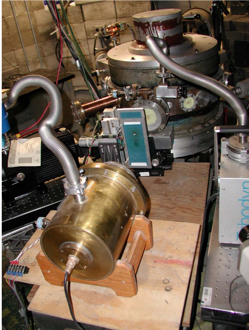
Figure 32. Beam path from SEM to the Faraday Cup.
