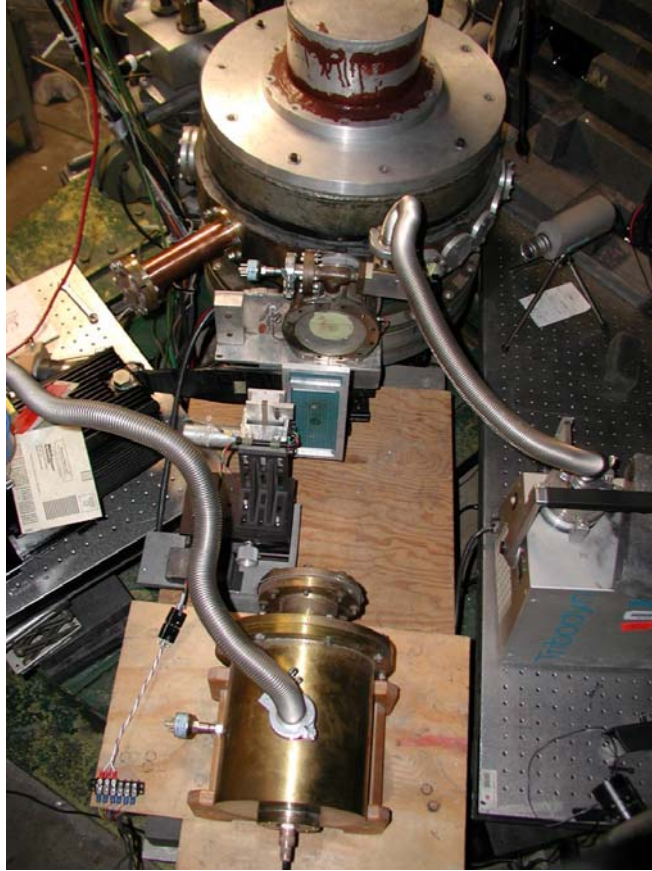
Figure 33. Top view of beam path. SEM at top, Faraday Cup at bottom.
