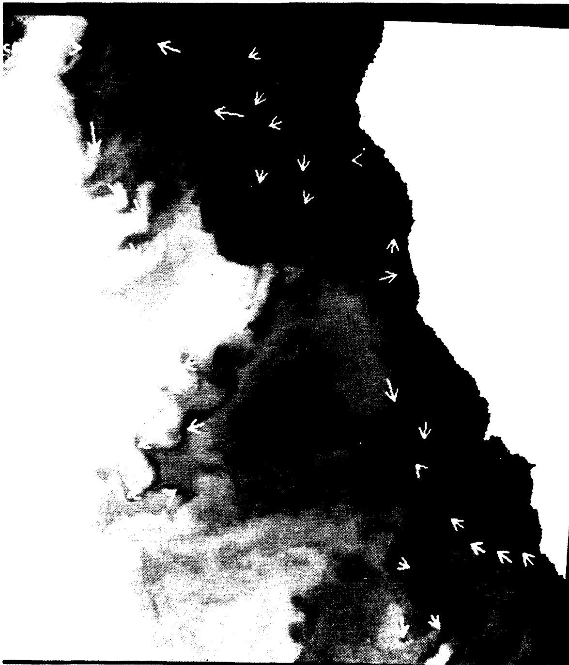
Figure E.11 Surface velocity vectors superimposed on channel 4 IR image from day 86315 (12:03 GMT). Vectors were calculated from day 86314 (21:55 GMT). \Delta t is ca. 14 hours. 10 cm/s scale in upper left corner. Land is masked white.
