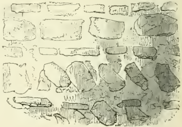
19. Rubble Masonry, Gundulph's Tower, called St. Leonard's, at Malling, Kent, A.D. 1070. The earliest Norman Keep in existence.
