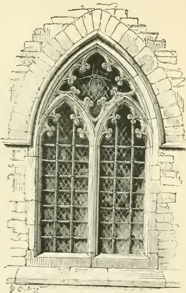
94. Solihull, Warwickshire, c. 1260. An early example of bar-tracery with ornamented cusps.
