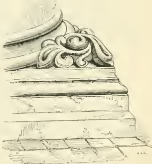
50. St Cross, Winchester, c. 1180. Late Norman Base and Foot-ornament.
