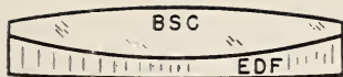
FIGURE 3. Cemented objective calculated in section 3 with appropriate thicknesses for a relative aperture of f/5 .
