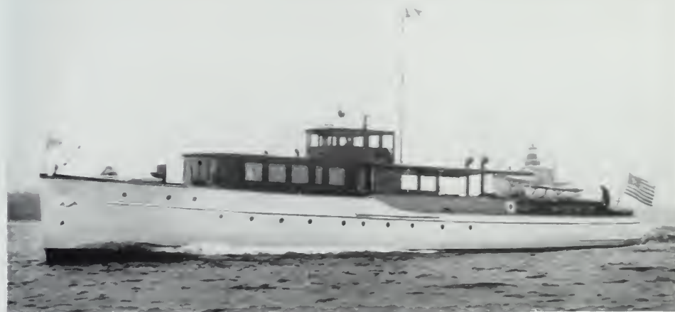
Among the fastest of Diesel-powered craft, Vixen, owned by Adolph M. Dick, Esq., of New York, made better than twenty miles an hour in her test spin. Three Speedway engines provide the power for this 110-footer which was designed and built by Consolidated
