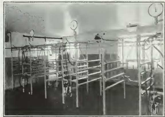
Special unit of six Loudon Combine Milking Stalls, entirely separated from the housing and feeding stalls, for sanitation, convenience and economy in handling the milking operation.
