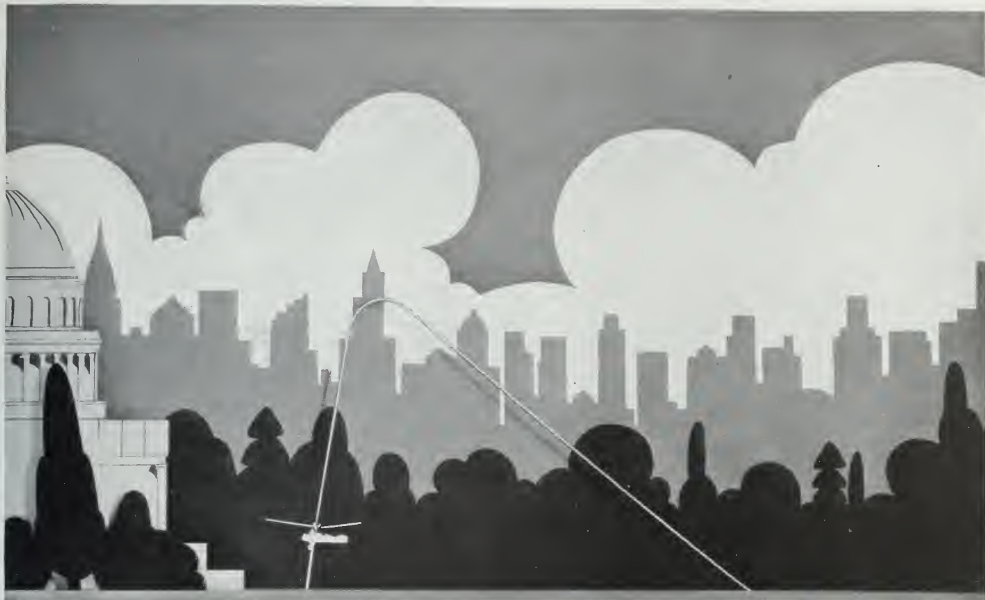
Reproduction of a chart showing safe vertical landing before an obstacle. In case the machine can not clear the obstruction, or the engine stops, the craft will land safely because the engine does not turn the sustaining rotor.
