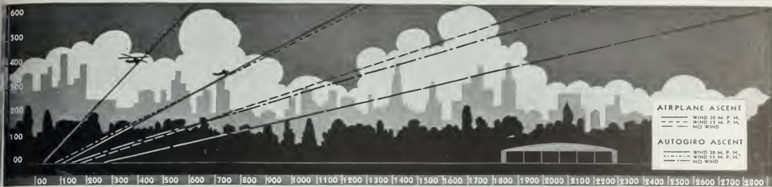
Photographic reproduction of a chart showing the steep angle of climb in a Pitcairn Autogiro under various wind conditions compared with an airplane of equal power
