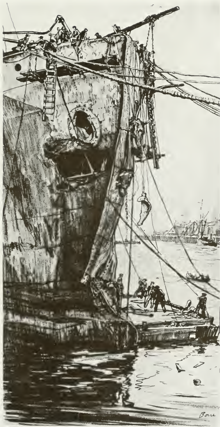
THE BOWS OF THE KISHU MARU DAMAGED BY COLLISION
