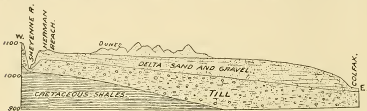
FIG. 13.—Section across the delta of the Sheyenne River. Horizontal scale, 6 miles to an inch
