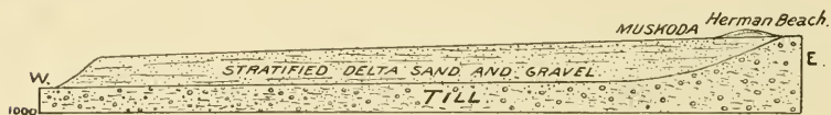
FIG. 11.—Section across the delta of the Buffalo River. Horizontal scale, one-half mile to an inch.
