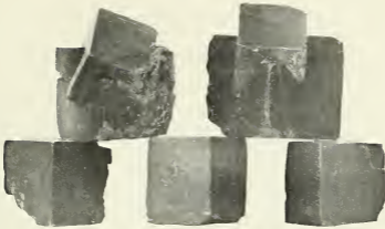
Limonitized, simple and twinned crystals of pyrite, from Gateway formation at summit of McGillivray range. Two-thirds natural size.
