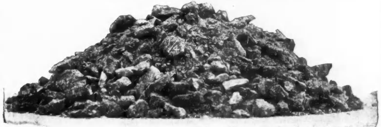
Direct product actual size from a ROLL JAW CRUSHER without screens
