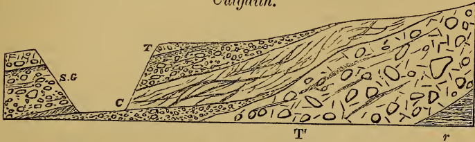
Fig. 3.—Section in the Settle and Carlisle Railway-cutting at Culgaith.
