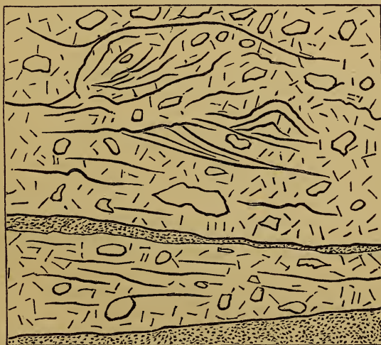
Irregularly stratified gutta-percha clays in lower till, with seams of soft sand. Length 4 ft.
