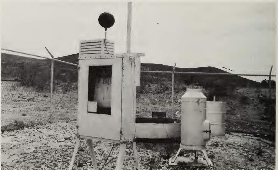
Rainfall, evaporation, and humidity are measured at this weather station on Walnut Gulch near Tombstone.
