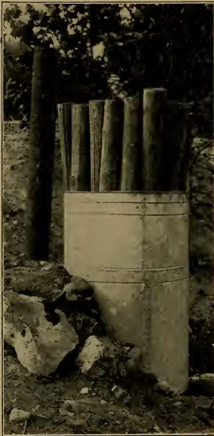
FIG. 55. — Single tank for treating posts.
