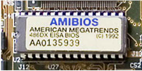
ROM BIOS firmware on a Baby AT motherboard
