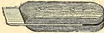
FIG. 100.—Knife for freezing microtome, made from the blade of a carpenter's plane.
