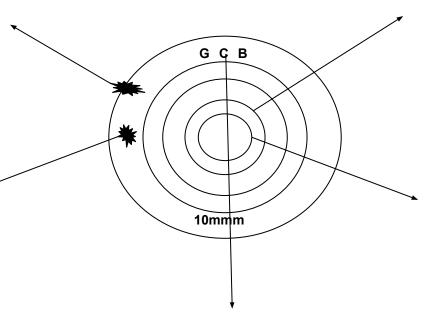
BreechBlock marking: (circular line) These markings are made by the force that pushes the cartridge backward against the breechblock when a bullet is fired and moving forward.
