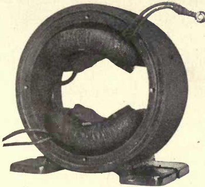
FIG. 68. Frame of a two-pole motor showing field coils and poles.
