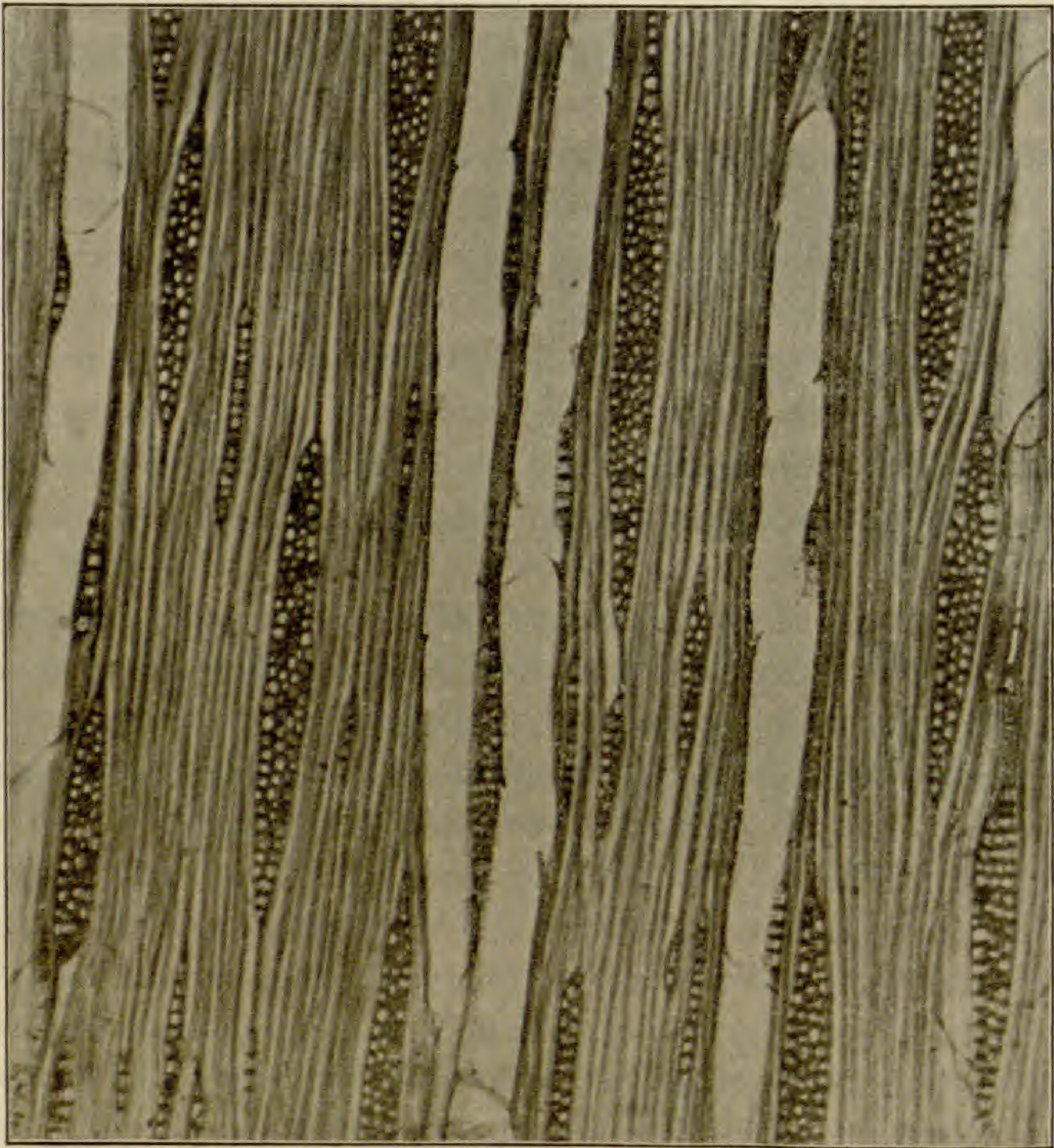
FIG. 1.— Maple wood, tangential section. Note the massive pith rays, and the large number of wood fibers.
