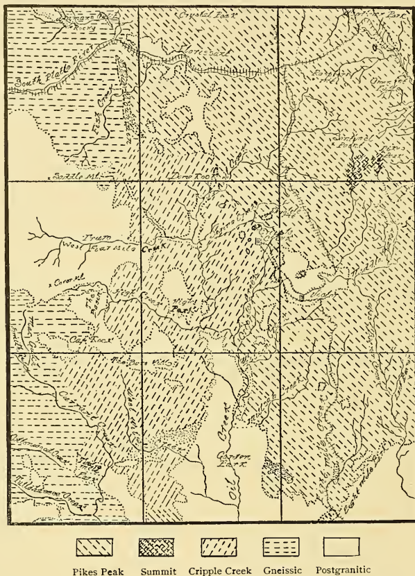
FIG. 4.—Sketch map showing the distribution of the various types of granite occurring in the Pikes Peak quadrangle.
