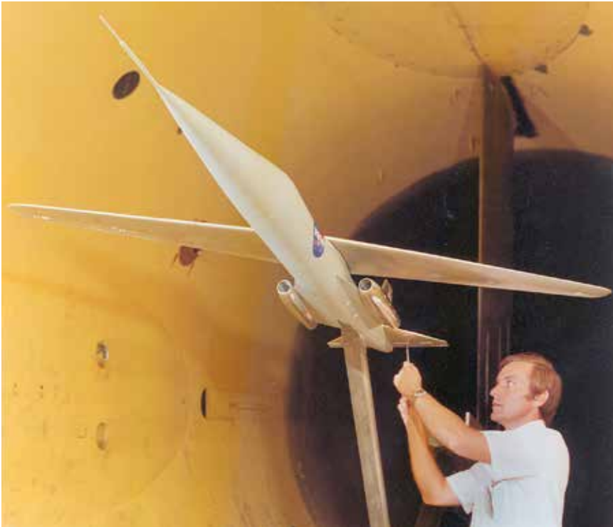
Ronald C. Smith of the NASA Ames Research Center with the AD-1 oblique-wing wind tunnel model. (NASA)
