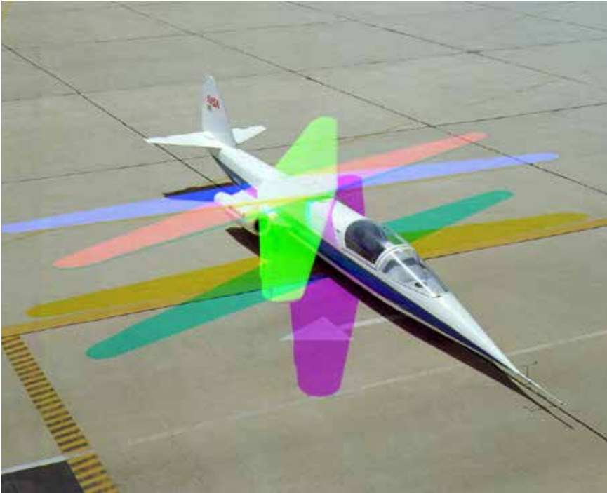
This time-lapse photograph shows three of the various sweep positions that the AD-1's unique oblique wing could assume. (NASA)
