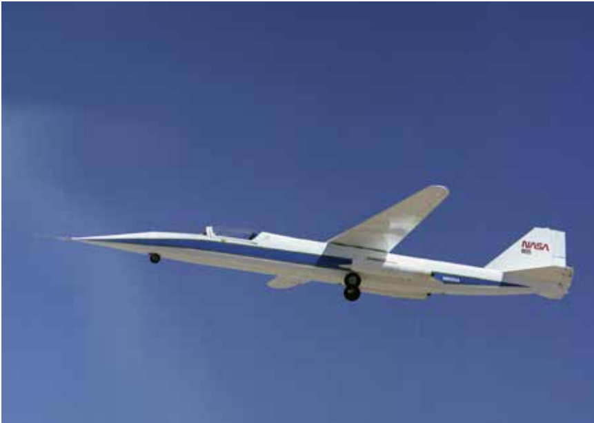
The AD-1 at 20-degree wing sweep, during its 13th flight, on April 25, 1980, for flutter clearance, piloted by Tom McMurtry. (NASA)
