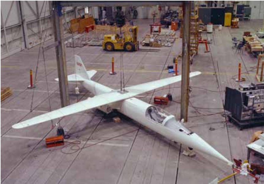
The AD-1 undergoing a ground vibration test at the Dryden Flight Research Facility, March 15, 1979. (NASA)
