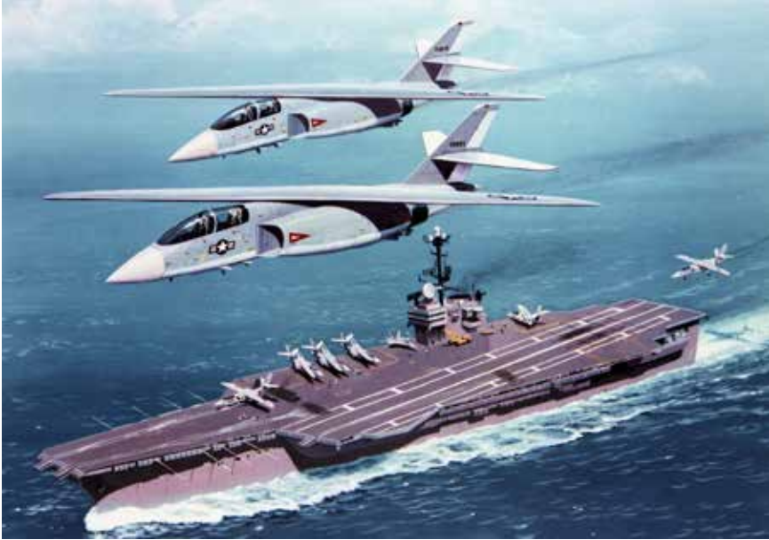
Rockwell concept for a Mach 2+ oblique-wing, twin-engine, two-seat, carrier-based, multimission fleet air defense fighter for the U.S. Navy's VFMX study effort, 1985. (NASA)
