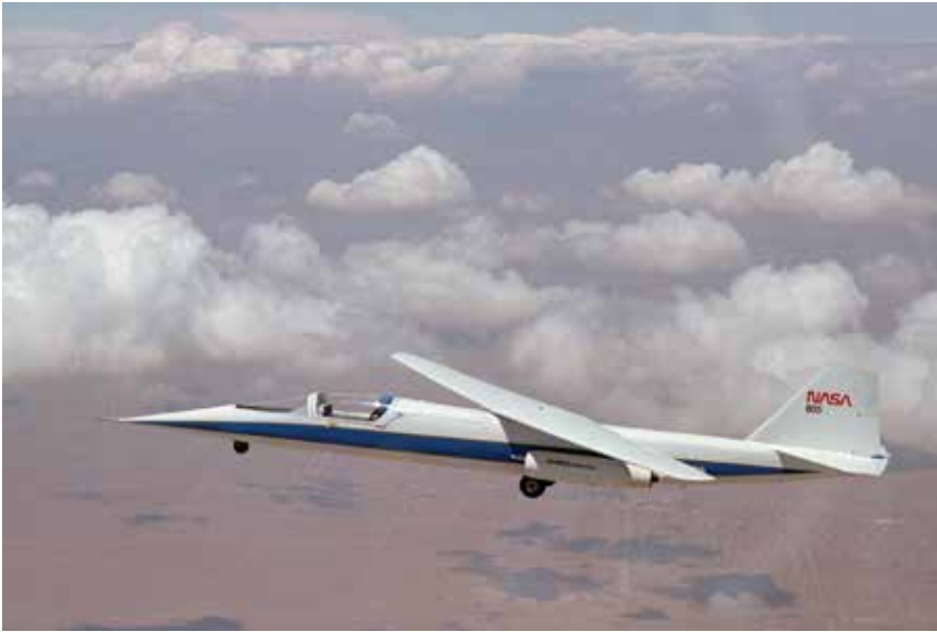
The AD-1 at 45-degree wing sweep, during its 14th flight, on May 28, 1980, for flutter clearance, piloted by Tom McMurtry. (NASA)
