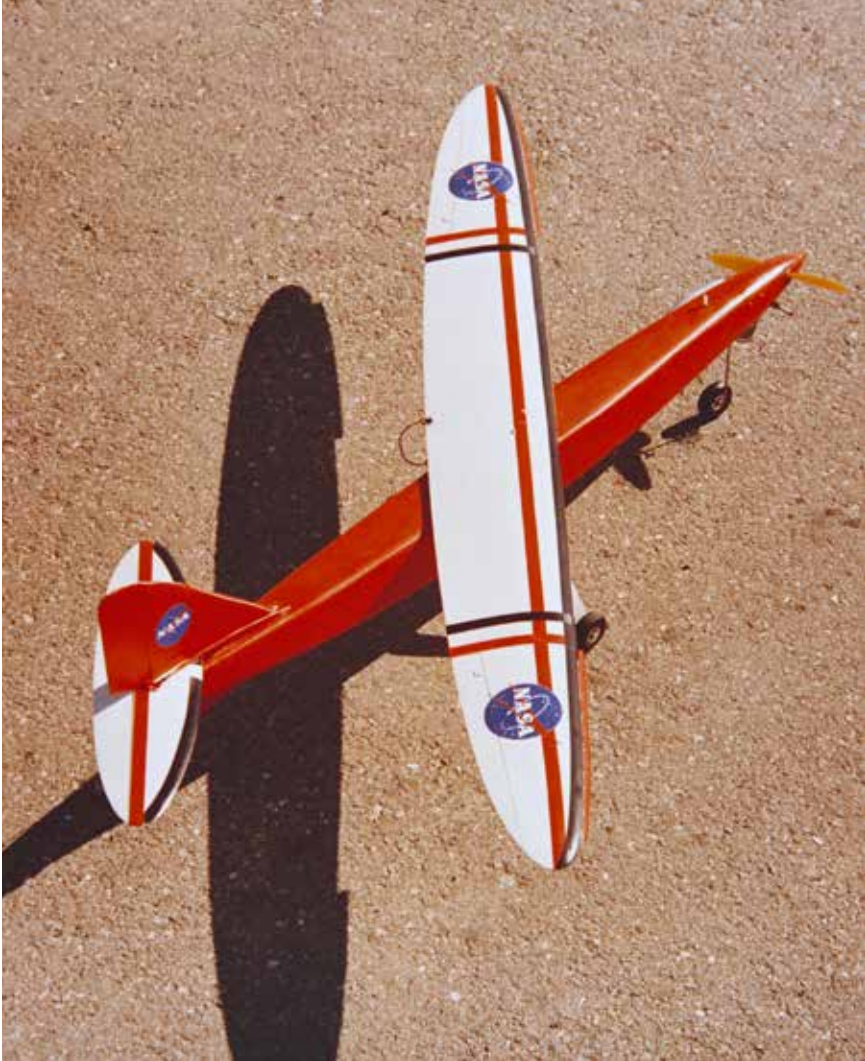
Jones-Gadeburg radio-controlled oblique-wing free-flight model. (NASA)
