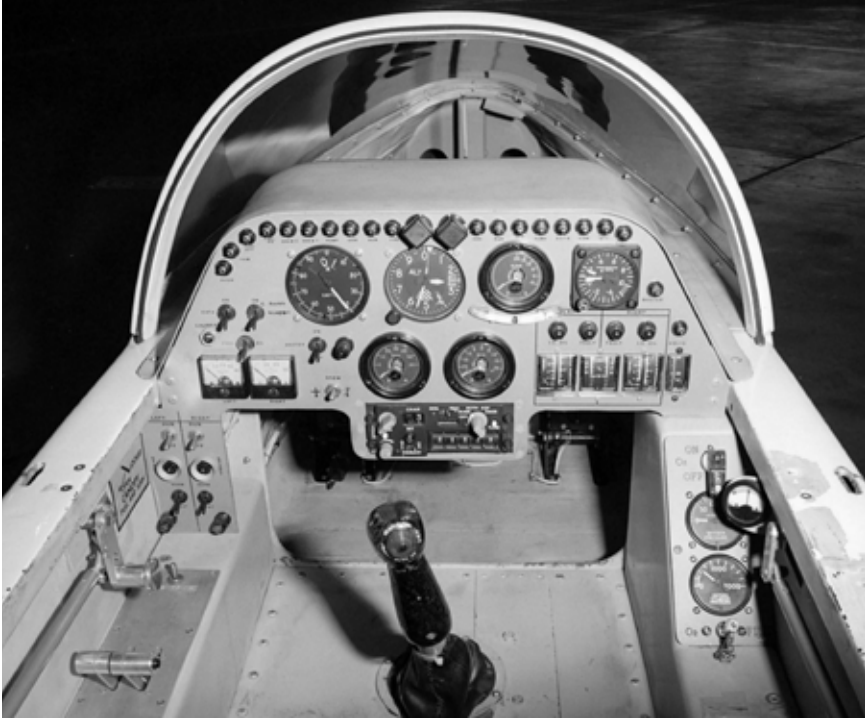
Cockpit and instrument panel of the AD-1 Oblique Wing Research Aircraft. The wing sweep "skew" gauge is center-left on the lower row of panel instruments; the sideslip gauge is center-right on the lower row; the angle-of-attack gauge is center-right on the top row. The dual-engine throttles are on the left side, and the dual-engine instruments are on the lower right side. Note as well the centerline control stick capped by a stabilizer-trim switch. (NASA)
