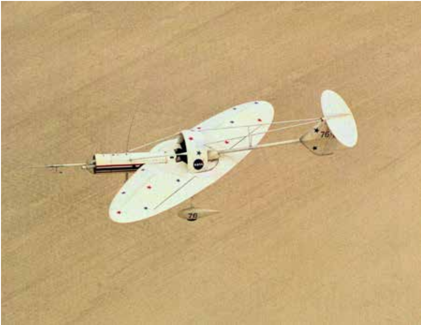
The OWRPRA (in long-tail configuration) in flight with its oblique wing in skewed position, 1976. Note its special bicentennial commemorative markings scheme. (NASA)
