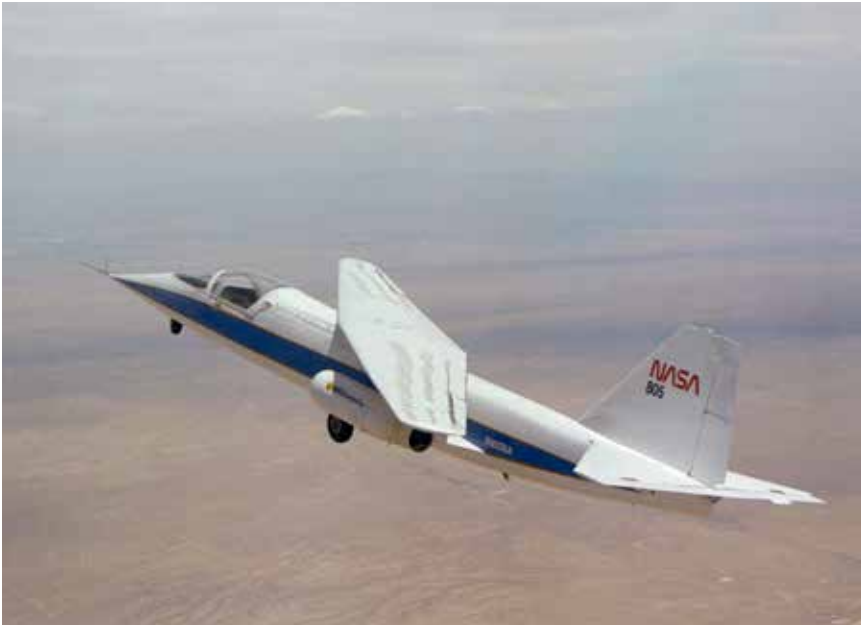
The AD-1 at 60-degree wing sweep, during its 32nd flight, on July 14, 1981, for flow visualization study (note the tufted wing), piloted by Fitz Fulton. (NASA)
