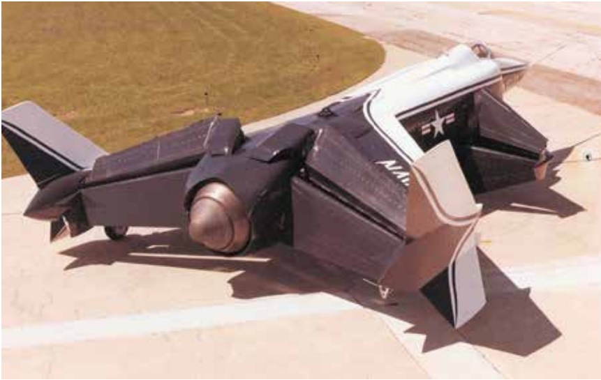
The North American–Rockwell XFV-12A augmented-wing V/STOL test bed at Columbus, OH, with its wing in VTOL configuration, 1978. (USN)
