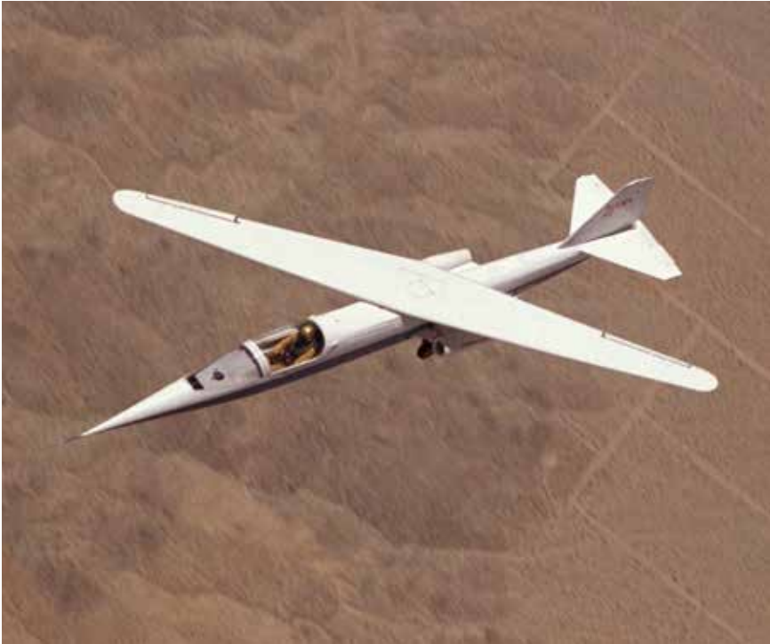
The AD-1 cruising over the Mojave in 1980 with its oblique wing set at a 60-degree sweep. (ASA)
