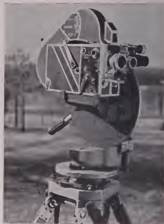
Above, left, the magazines can be changed without dismantling the camera. Above, right, (front quarter view). The winding crank and other camera controls are easily accessible. Note the dovetail clamps which hold the front attachments when desired.
