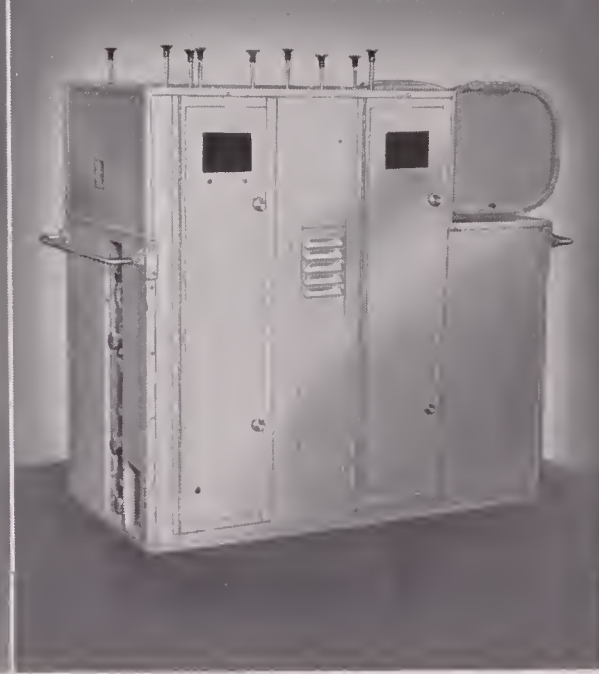
Processor showing dry-box side as for operation.
