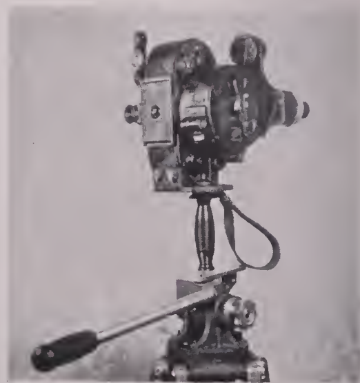
Eyemo turret with prismatic focusing magnifier and alignment gauge removed, showing ground glass cover, ratchet winding key, handle and strap in place. The tripod was merely used to hold camera upright while being photographed.
