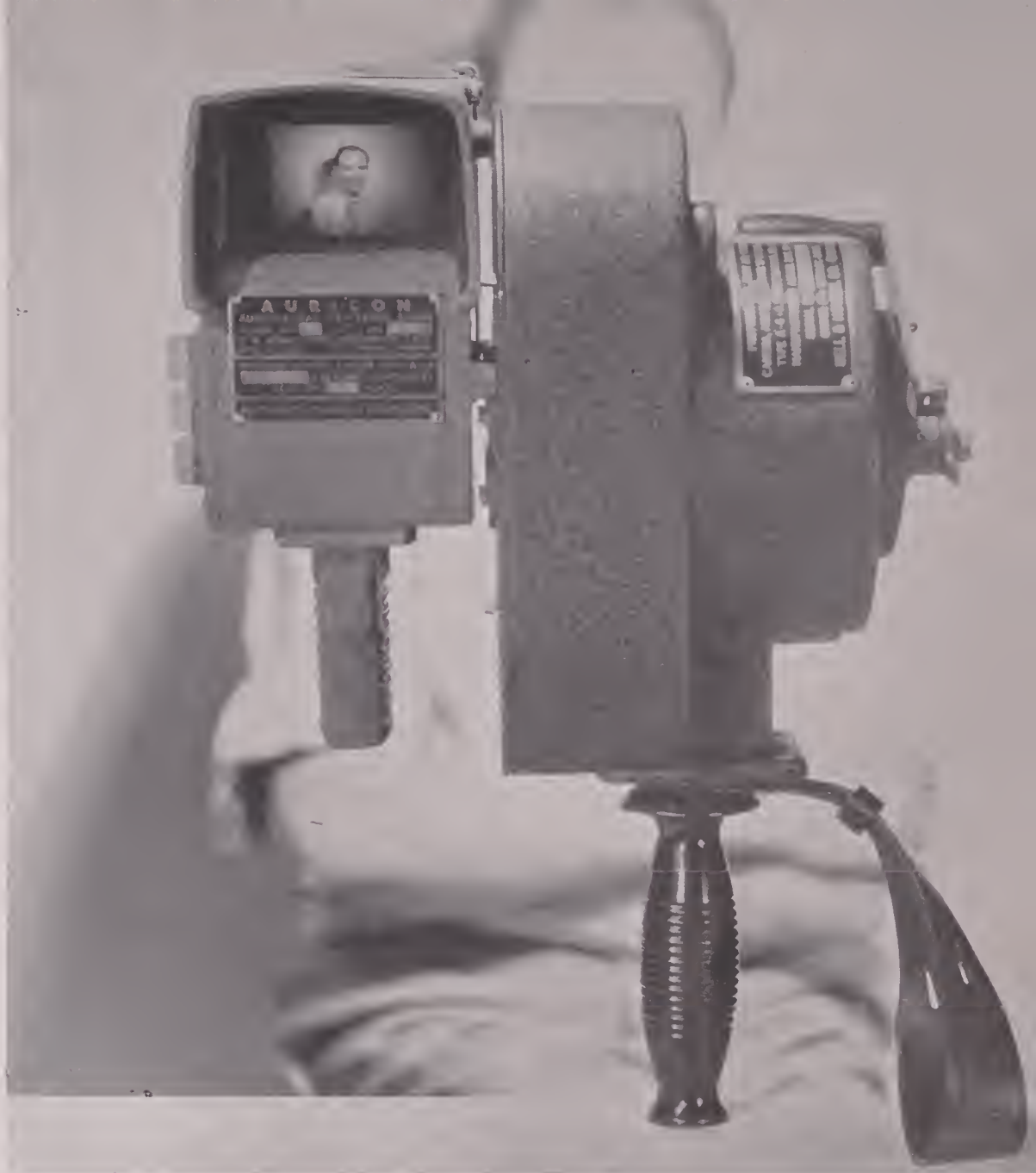
Above, Unretouched photograph looking through the new Auricon Finder, showing large needle-sharp image, upright and correct right to left. Focusing this image in the finder automatically corrects parallax and also indicates distance from camera to subject being photographed.
