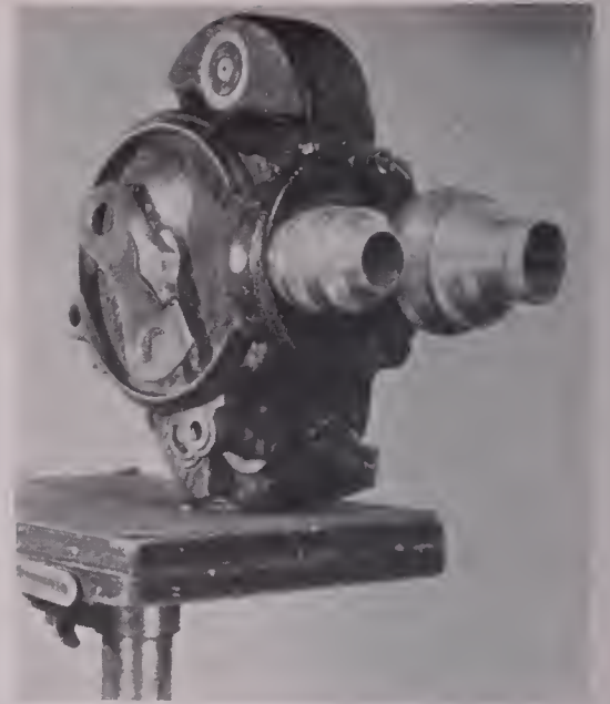
Left, Richard Thomas, inventor of Thomascolor checking a new Thomascolor lens on a standard motion picture camera. Above, a Bell & Howell 16 mm camera equipped with Thomascolor 1-inch and 2-inch lens mounts, on a turret.
