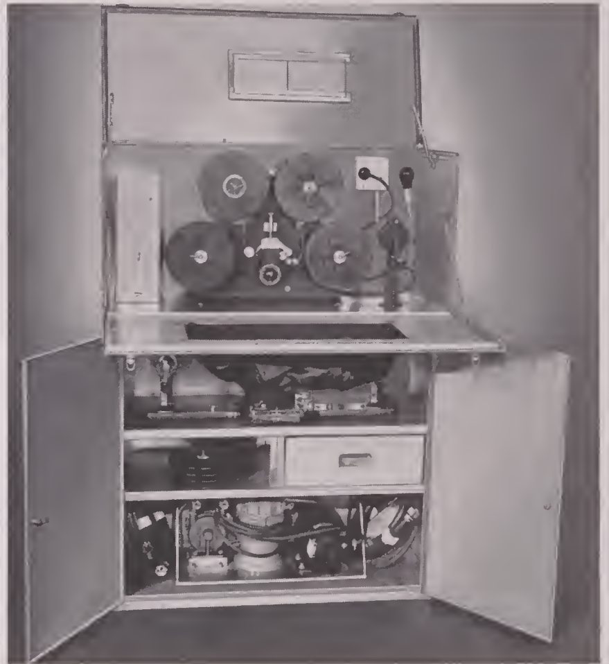
Darkroom as packed for shipment but showing printer threaded as for operation.
