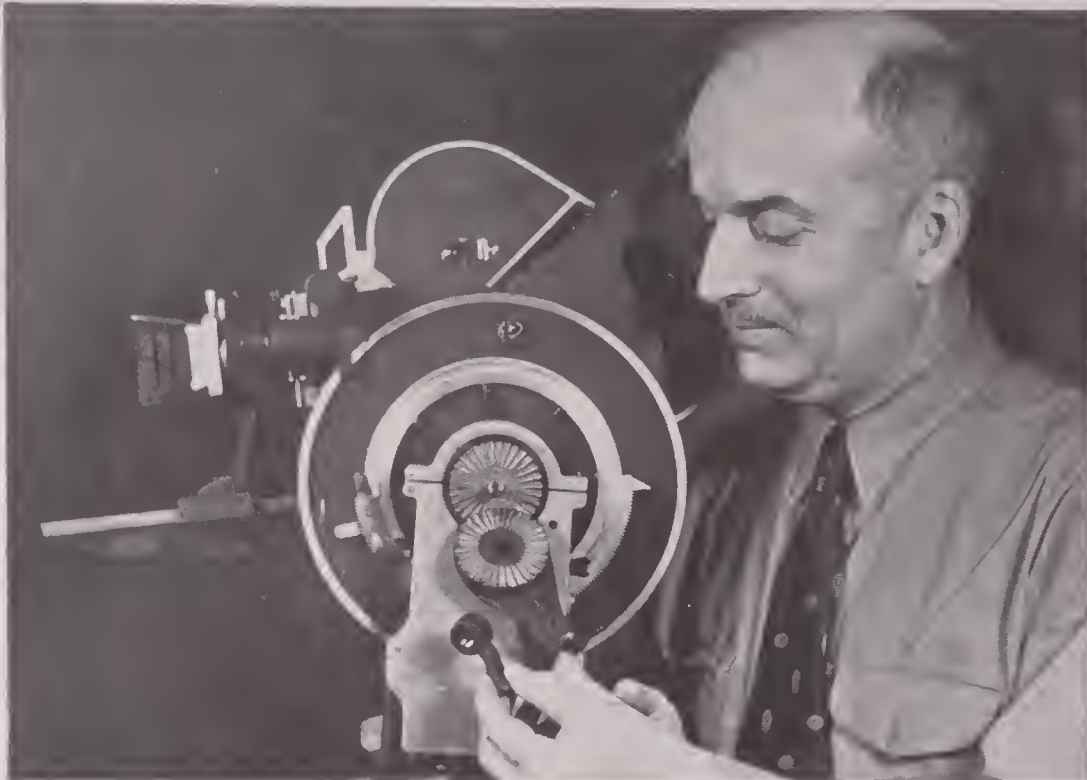
Above, a pair of serrated discs allow the stick to be clamped at any desired angle; and being installed to the left of the camera mount, it cannot interfere with the tripod top.
