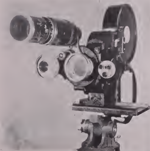
Eyemo 71C-A showing pola screen and filter holders on 1" f.2, 2" f.2/5 and 6 1/4" f.3/5 lenses.
