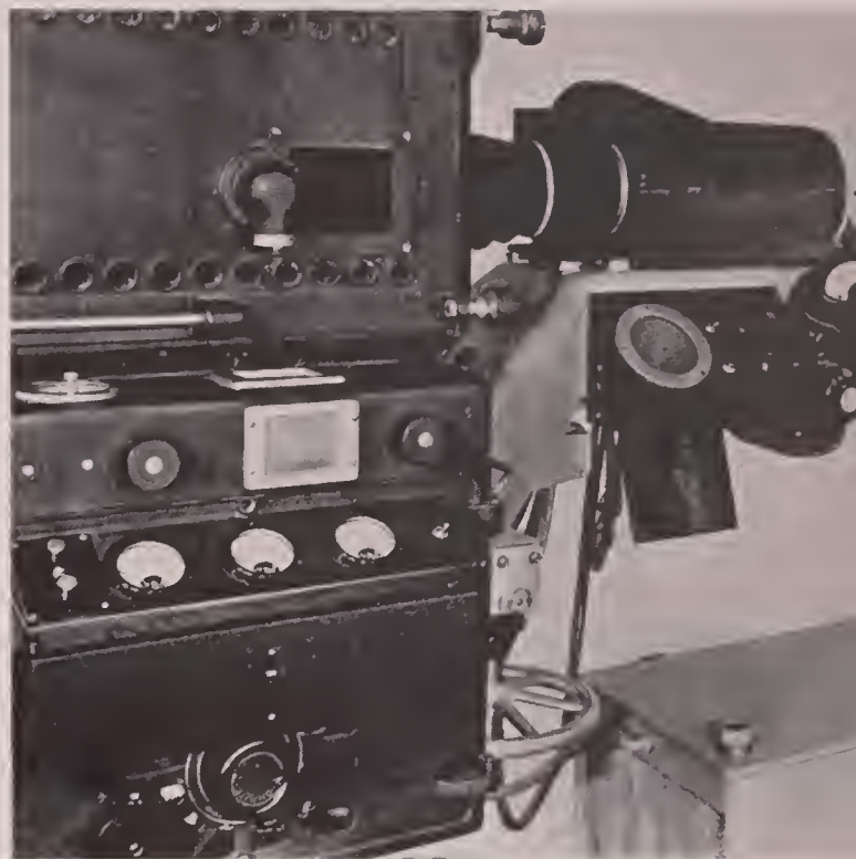
Top left: Fig. 2. Paramount transparency stereopticon cooling unit consisting of radiation units for water-cell and lamp water circulation.
