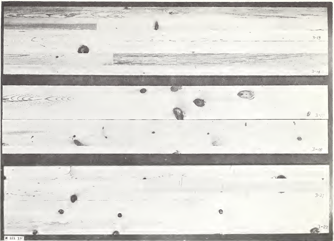
Figure U-6(above). — Lumber panels with a wide range of quality used for paper-over- laid siding.
