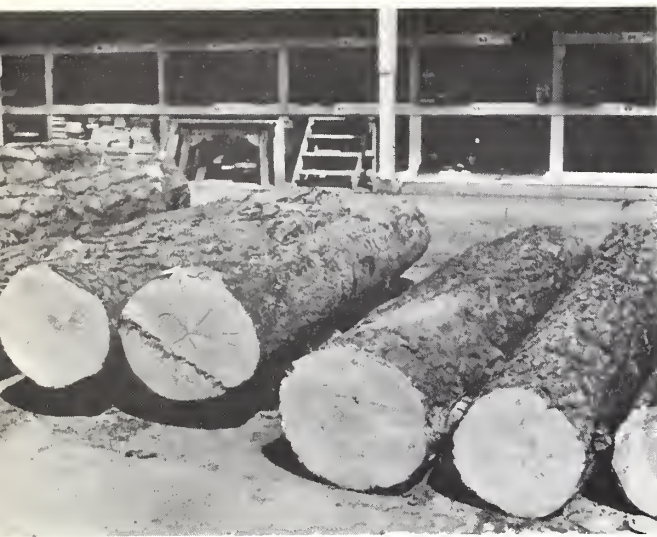
Figure U-1(left). – Low-grade ponderosa pine logs used in veneer and plywood evaluations.
