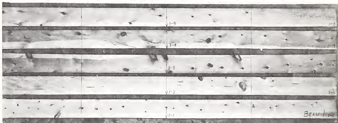
Figure U-3(above). — Quality and orientation of laminations in test beam No. 1.
