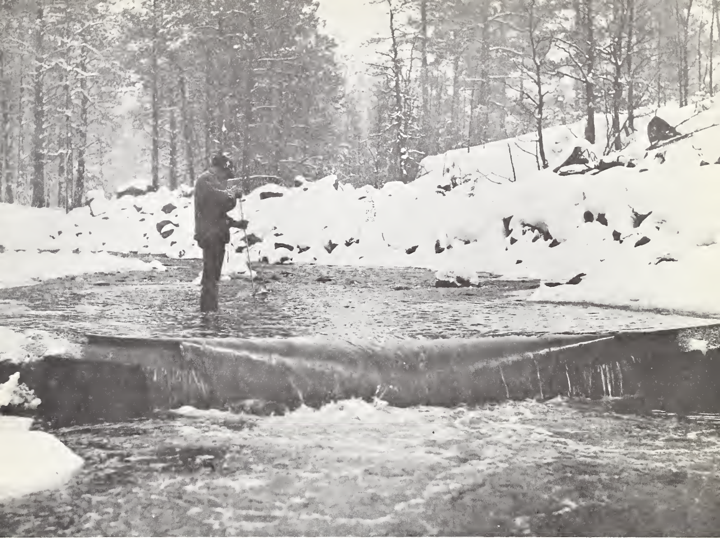
Figure W-17. - Current meter measurements at Bar M stream gage. The discharge was about 10 second-feet.
