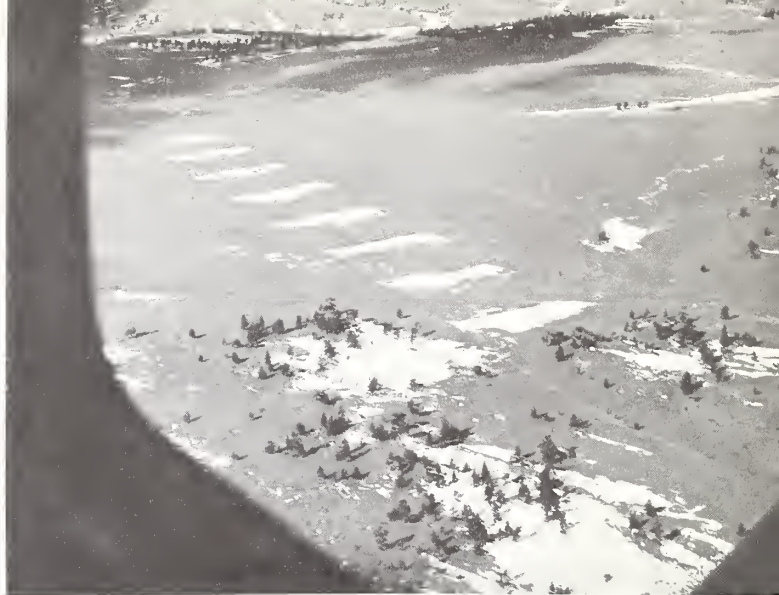
Figure W-7. — The importance of wind barriers for holding snow is shown by this aerial view of a snow-fence spacing trial on Pole Mountain, Wyoming. The picture was taken on February 7 when the accumulation was about half the maximum finally reached on March 22.
