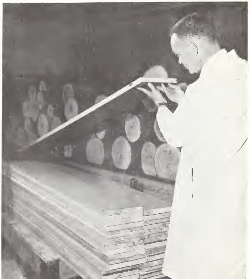
Figure U-7(right.) — Paper-overlaid siding panels ready to be re- sawn into two pieces of bevel siding. Double tongue-and-groove feature provides for tongues and grooves on individual resawn boards.
