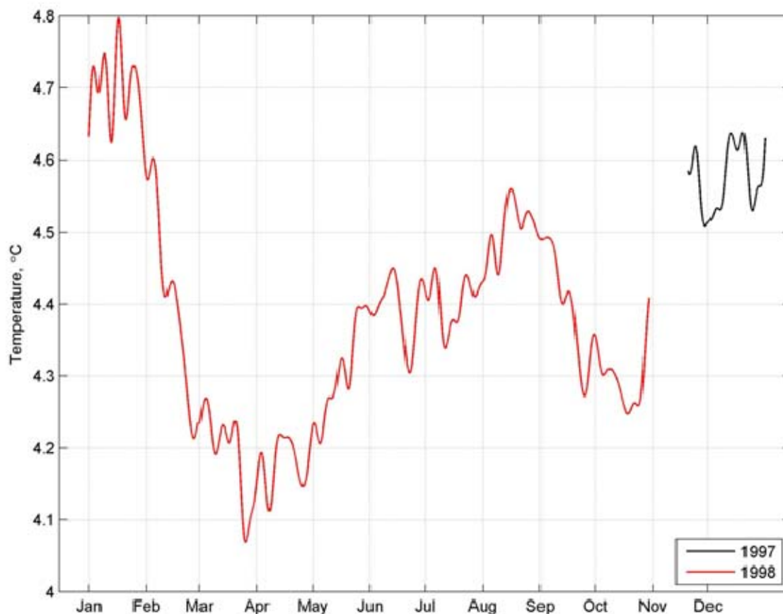
Figure D9. Temperature time series at 800 m at mooring R1. Temperatures were smoothed using a Butterworth filter that cut off periods less than one week.
